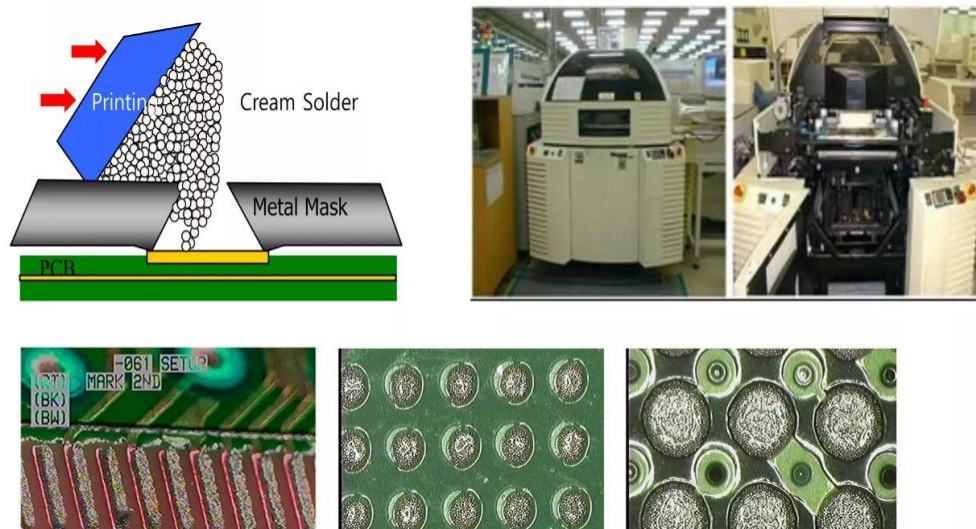
Gambar 11. Proses Printing Solder Paste
